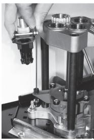
• Install bullet seating die and feeder assembly into position so action rod is close to vertical.
