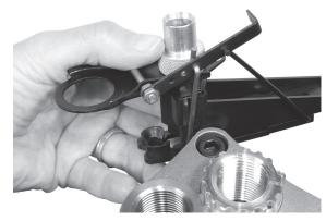
Slide down action rod and bullet feed assembly into the friction actuator.
